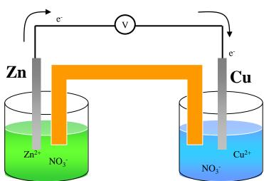
Anode / anode solution // cathode solution / Cathode
